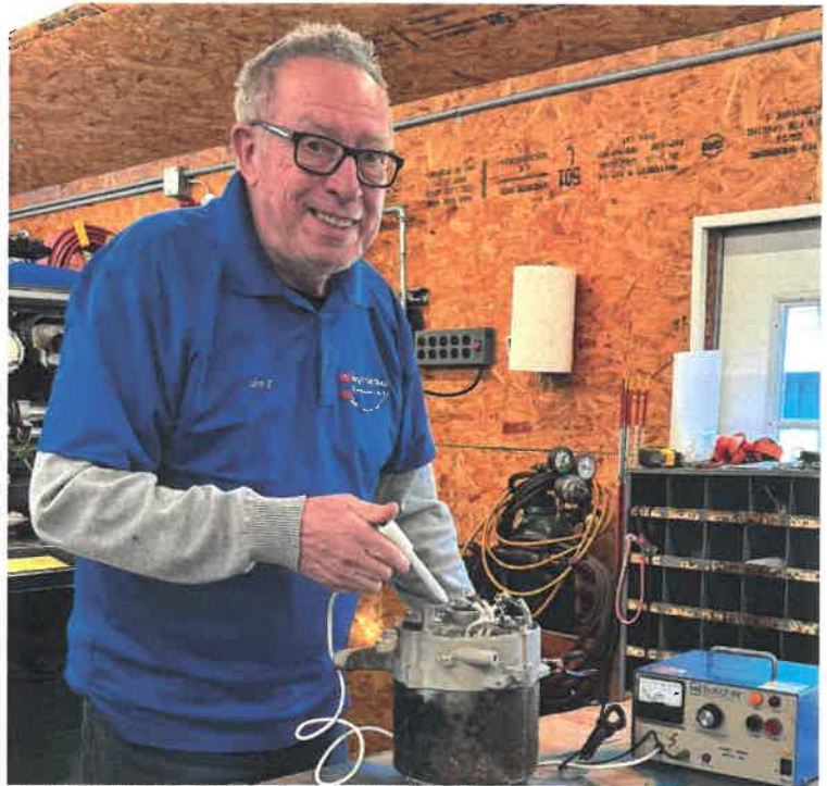
Jim Kocmoud performs high-potential testing of a generator winding.
